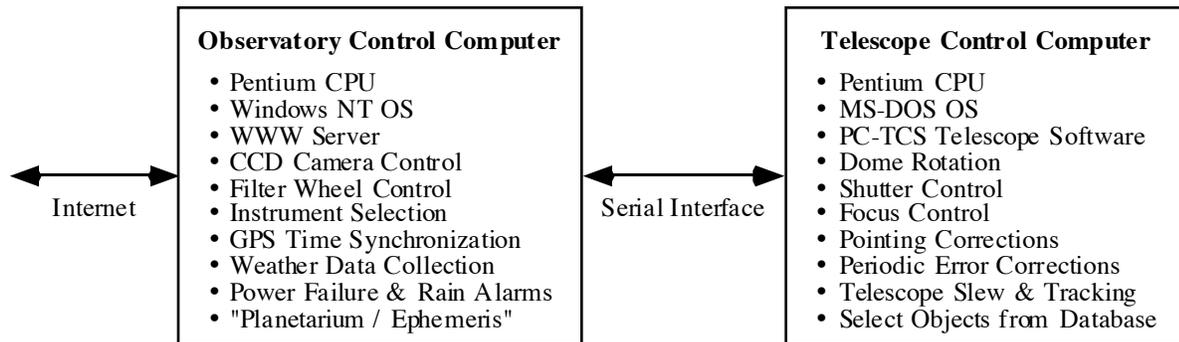
**Figure 3:** Schematic of observatory control system and high level functions.
