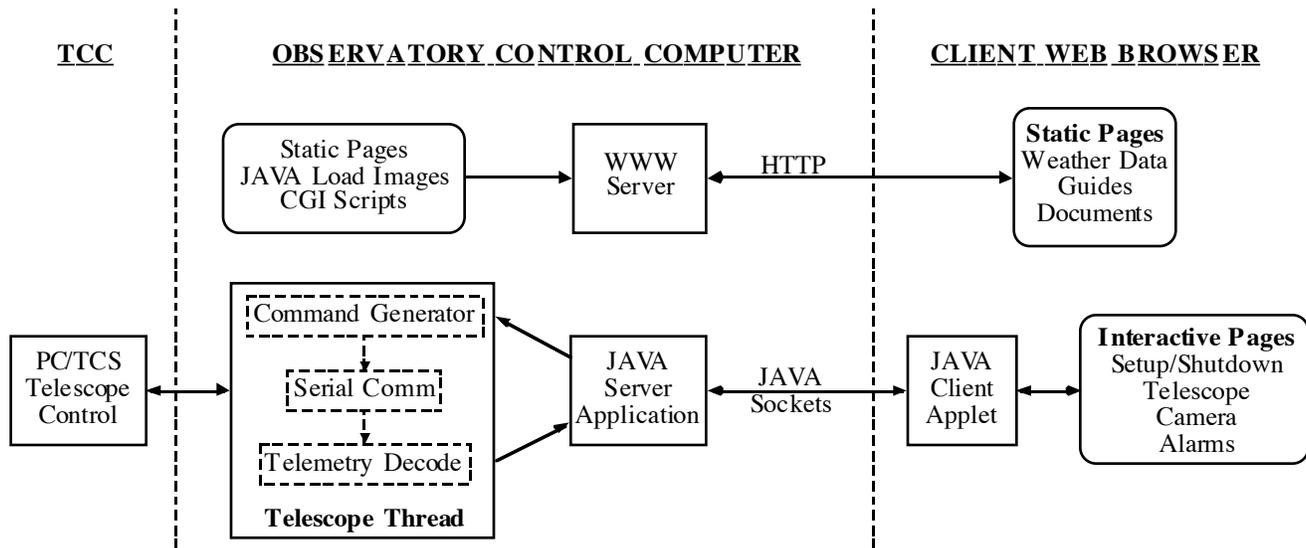
Figure 4: Remote telescope control processes and data flow schematic.
