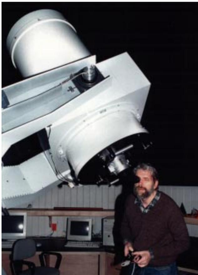
**Figure 2:** The 20" f/8.1 RC telescope and control computers located on the 2nd floor of the facility.
