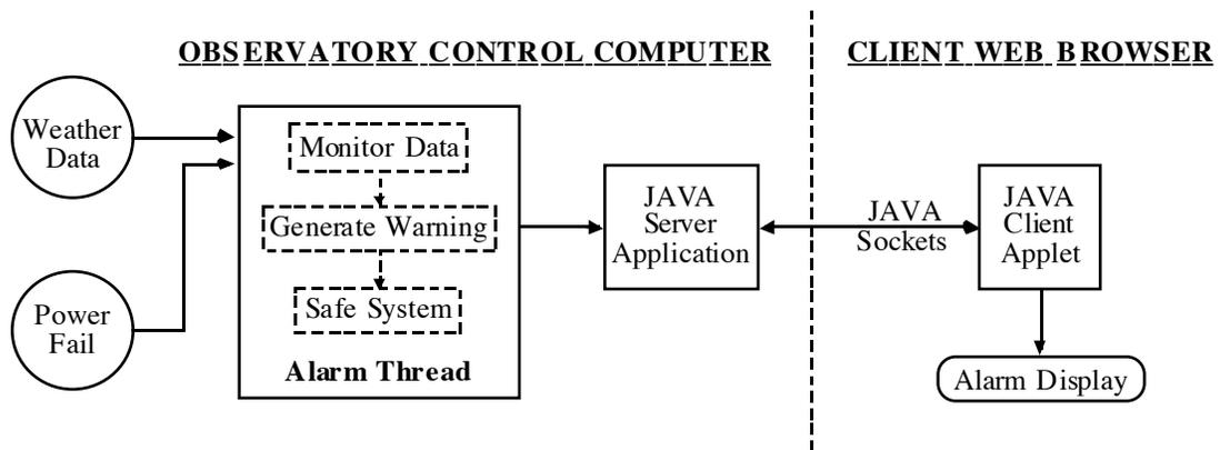
Figure 6: Alarm monitoring processes and data flow.
