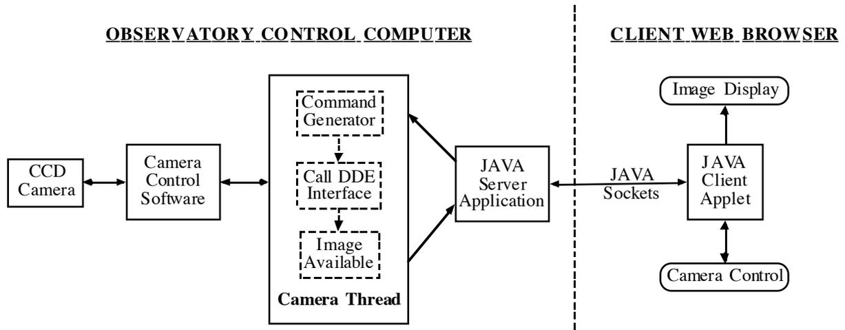
Figure 5: Remote camera control diagram of the processes and data flow.
